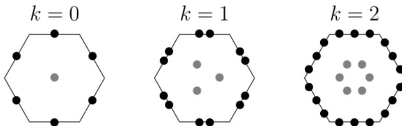
Ex: Degrees of Freedom (DOFs) for the **scalar case** using the **standard HHO** with hexagonal cells.
